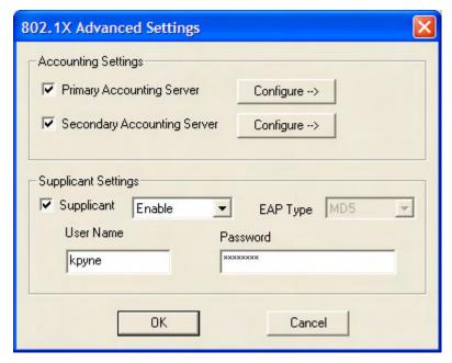
Primary and secondary accounting servers are similar to the settings for RADIUS servers. The supplicant settings let you configure the IntelliJack as a supplicant to an 802.1X-enabled upstream switch. To enable this option, select the box next to Supplicant. When you do, the other fields on the screen will become active. You can enter a Supplicant User Name and Password as well as an EAP Type setting. MD5 is the only EAP type that the IntelliJack currently supports.
